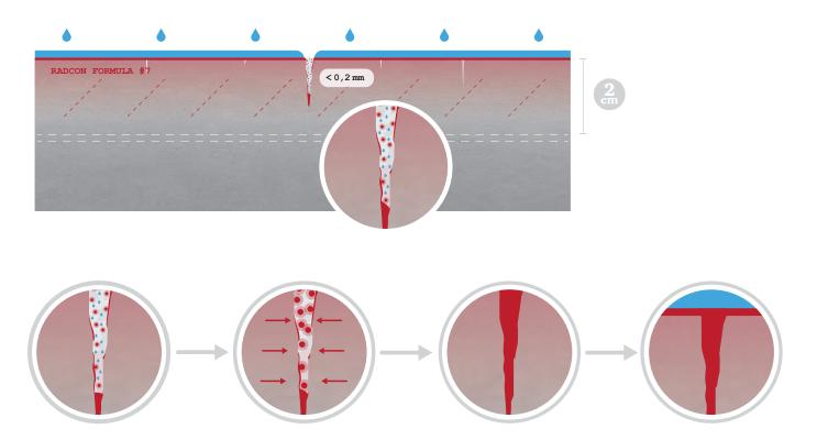
Unsealed concrete surfaces showing cracks up to 2mm can be fully sealed with Radcon Formula #7®.
