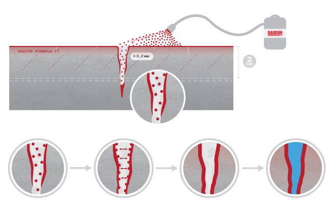
Concrete surface with hairline cracks treated with Radcon Formula #7 remains 100% waterproof. The cracks will be completely closed by the expansion of Radcon Formula #7®.
