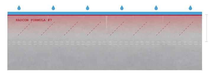
Concrete surfaces treated with Radcon Formula  $\#7^{\$}$  with cracks from 0.2 to 2 mm are 100% waterproof. The cracks will be completely slowly closed by the expansion of Radcon Formula  $\#7^{\$}$ .
