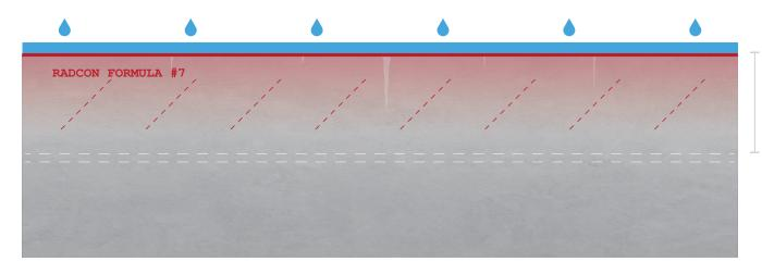
Concrete surfaces treated with Radcon Formula  $\#7^{\$}$  with cracks from 0.2 to 2 mm are 100% waterproof. The cracks will be completely slowly closed by the expansion of Radcon Formula  $\#7^{\$}$ .
